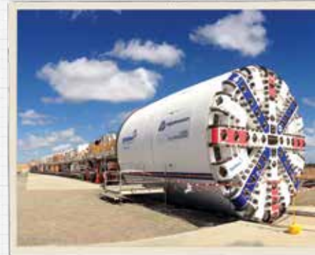
The Robbins Crossover (XRE) TBM pictured here is at the forefront of a trend for efficient machines that can operate in mixed ground conditions.
